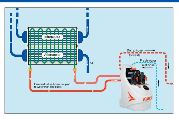
Scalebreaker C40 FWF with fresh water flushing facility
